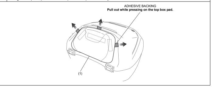
4. Applying adequate pressure of 5 kgf (50 N) to the attached top box pad, and then release the adequate pressure and leave the top box pad for 10 minutes to stabilize the fitting of the adhesive surface.
