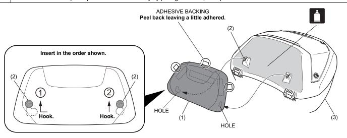
Install as shown.Align the top box pad with the shape of the top box securely.
